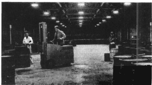
In one warehouse, 55 gal. drums of paint are stored. Electric trucks, which can lift to a height of 7 feet, facilitate stacking and quick transportation of the drums. George W. Corbell, checks the stock while Roy L. Coston manipulates the truck. (Right) Lee Wafford, guard.
