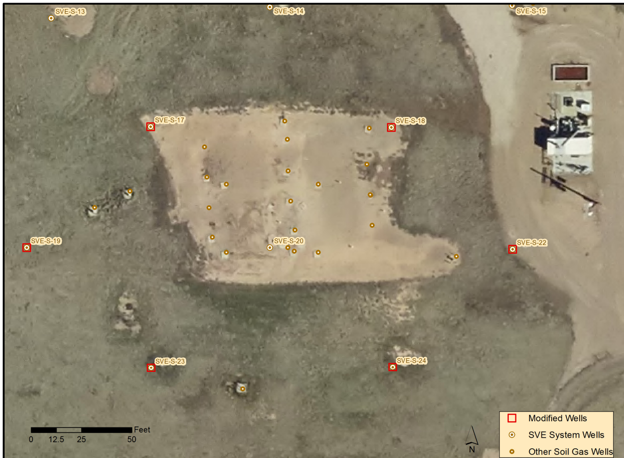
Figure 1-4. Burning Ground SVE System Wells and Modifications
