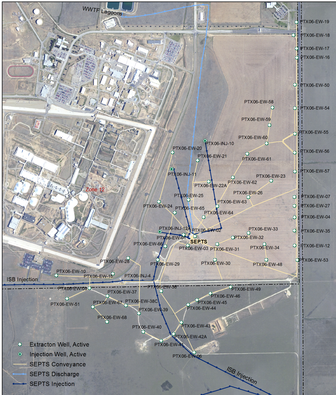
Figure 3-31. SEPTS Extraction Wells and Conveyance Lines
