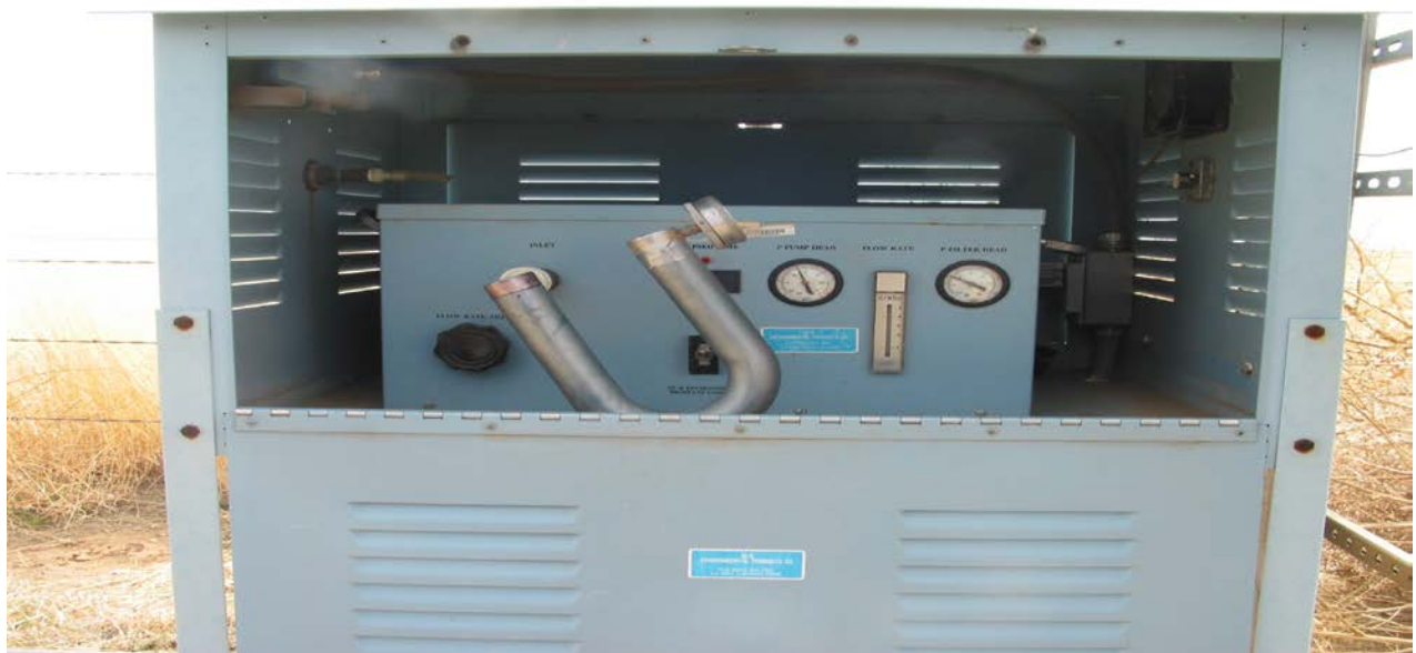
Figure 5.4 – Low-Volume Sampling Apparatus
