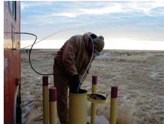
Sampling technician connecting sample lines at the wellhead.
