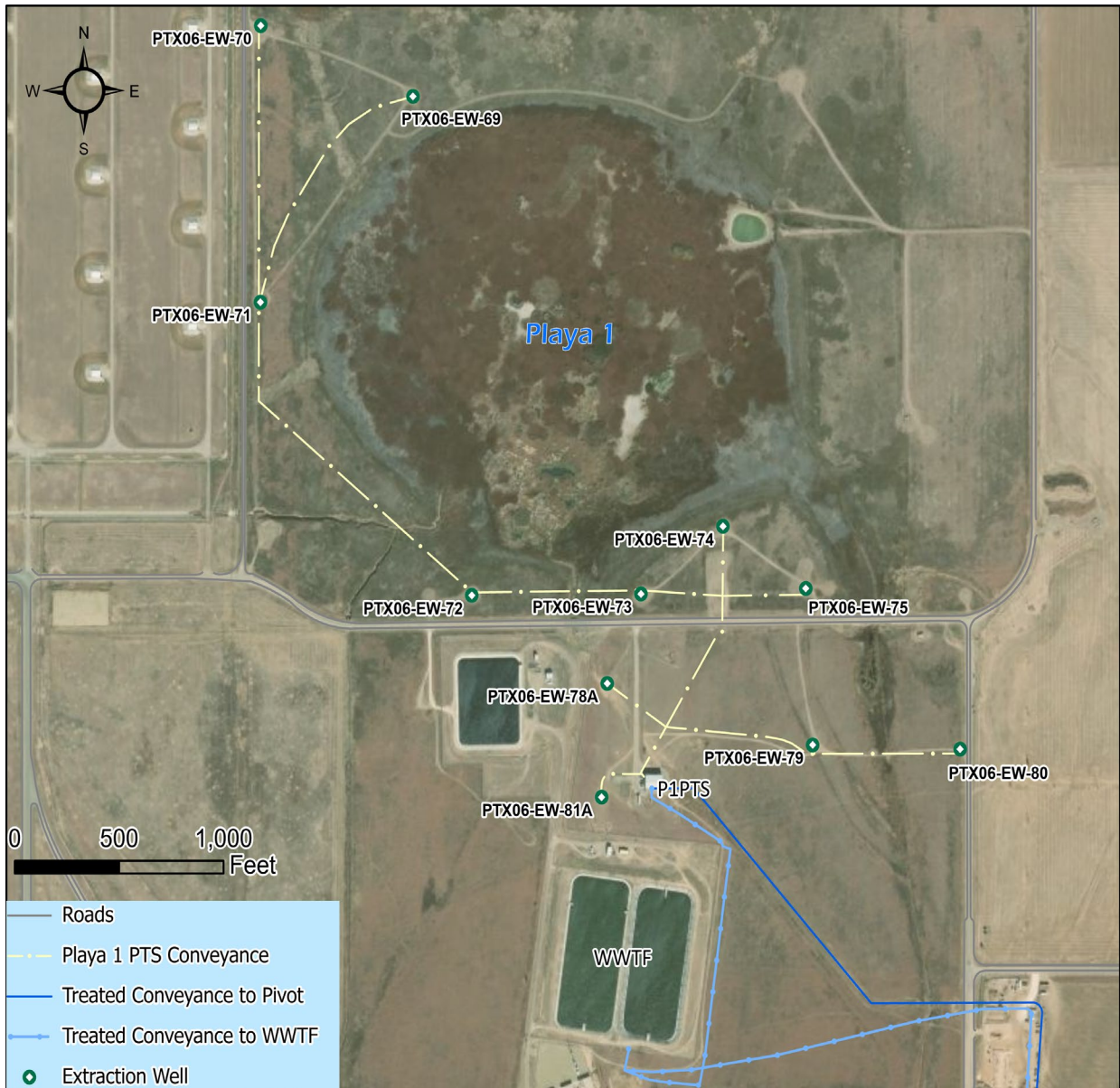
Fig. 1-6. P1PTS wells and conveyance lines.
